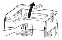
2. With an LED lens cleaner or soft cloth, gently wipe each of the four heads (1). Move the cleaner as shown, using a clean section of the cleaner with each pass. Be careful not to damage the guards (2).
